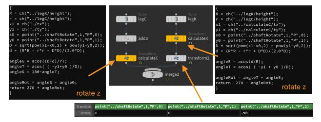
The rods start in an "L" shape at the origin, with leg K vertical and leg C horizontal. The transform node moves rod K to point X and rotates it to meet with rod C at point U.
