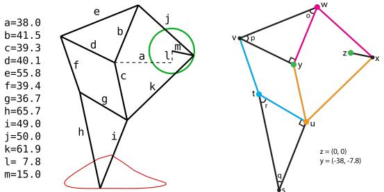
The rods must each be a specific length (Jansen's "Holy Numbers"), seen in the diagram on the left. In addition, points Y and Z and angles O, P, Q, R, and the right angles are fixed.
